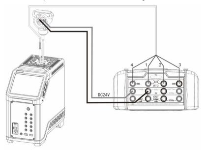
Figure 19 Temperature transmitter with sensor
