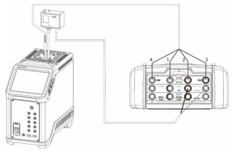
Figure 21 Temperature switch with sensor
