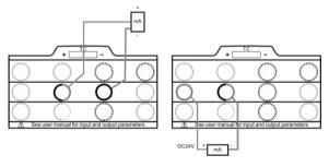
Figure 7 Current Measurement
