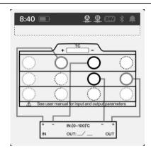
Figure 20 Temperature switch
