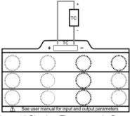
Figure 15 Simulate Thermocouple Output
