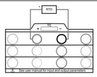
Figure 16 Simulate RTD Output Table 15 RTD Output Settings
